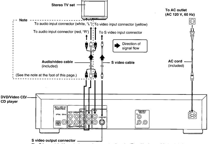
The S (separate) video output connector separates the color (C) and luminance (Y) signals before transmitting them to the TV set in order to achieve a sharper picture.
